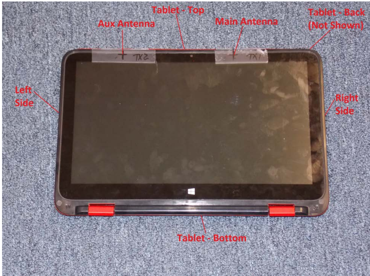
Test Positions and Antenna Locations
