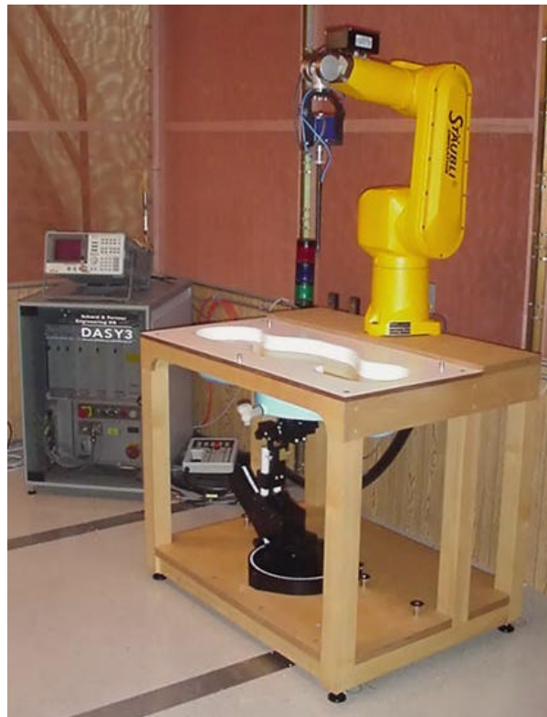
Fig. 1. DASY3 SAR Measurement System
