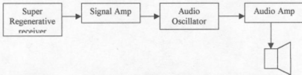
The super regenerative receiver recovers the 600Hz pulse from the RF. The signal is amplified and rectified to trigger the audio oscillator to produce an ultrasonic tone which is then amplified and sent to the speaker.
