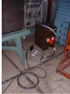
General Test Setup: Conducted Emissions
