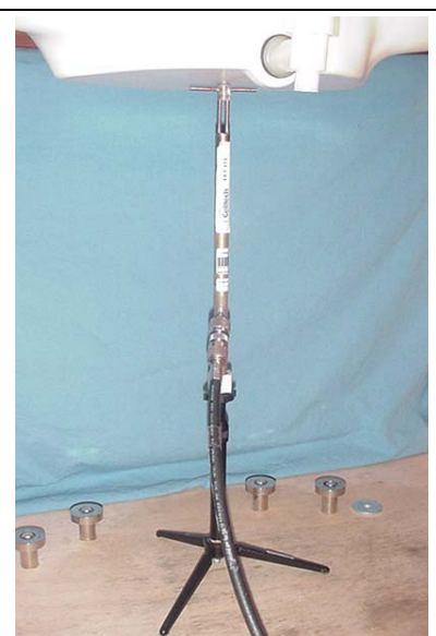
1900 MHz Validation Dipole Setup
