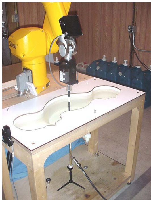
DASY4 System with SAM Phantom and validation dipole
