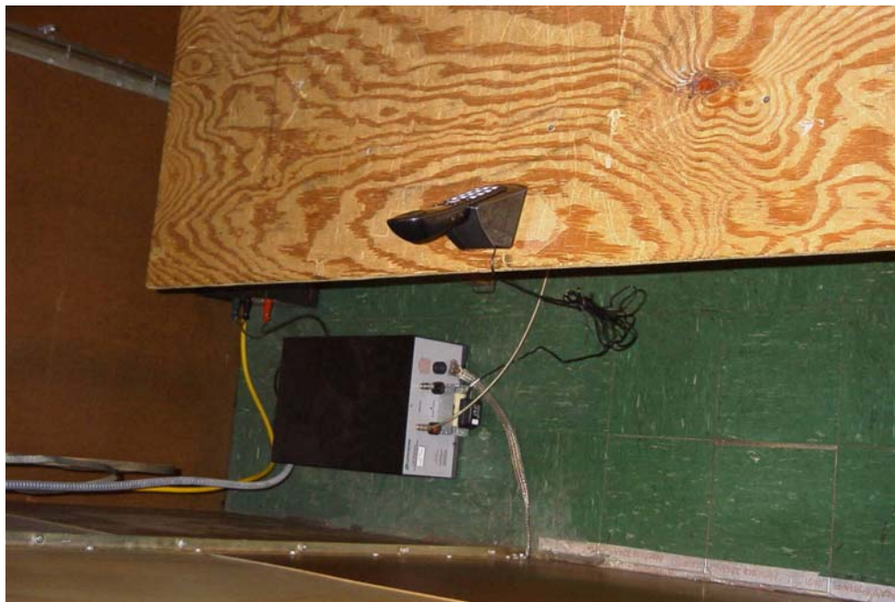
Powerline Conducted Test Set Up (Handset On Charger)
