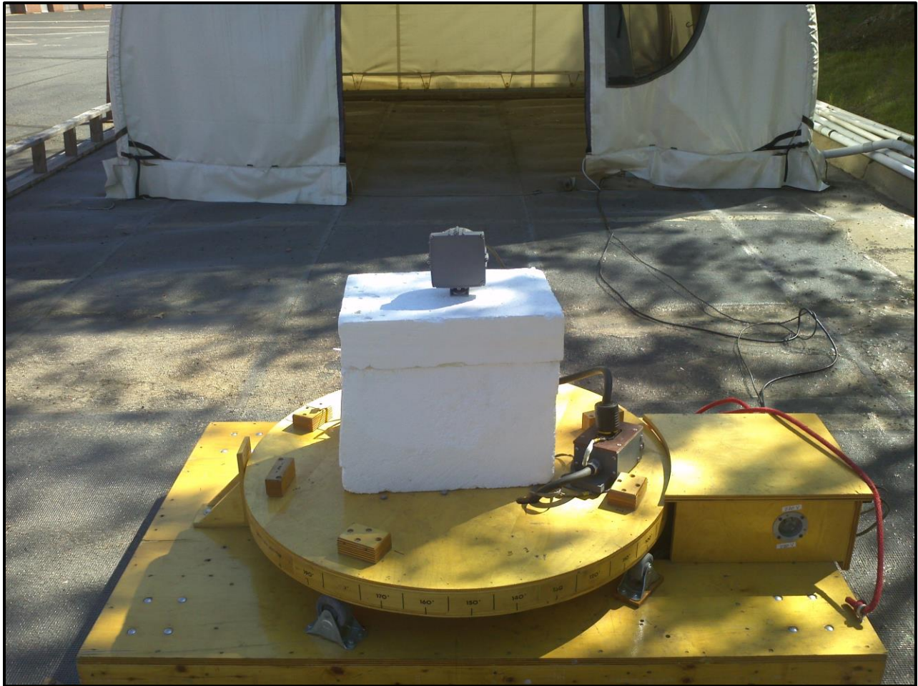
Photograph 2: Radiated Emissions - Front View
