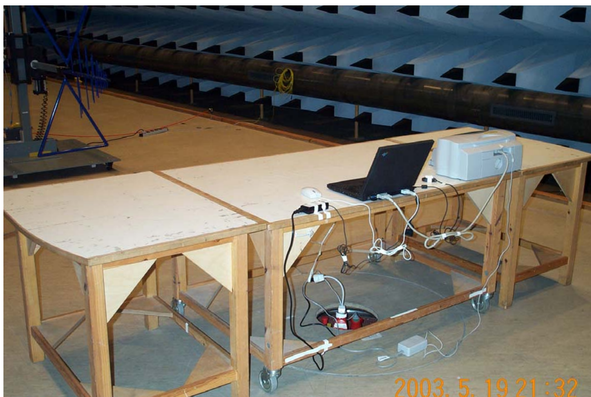
Photo A3.2 Radiated electromagnetic field measurement.
