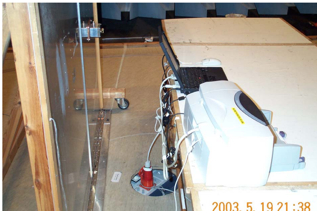
Photo A2.3 AC mains conducted emission measurement.
