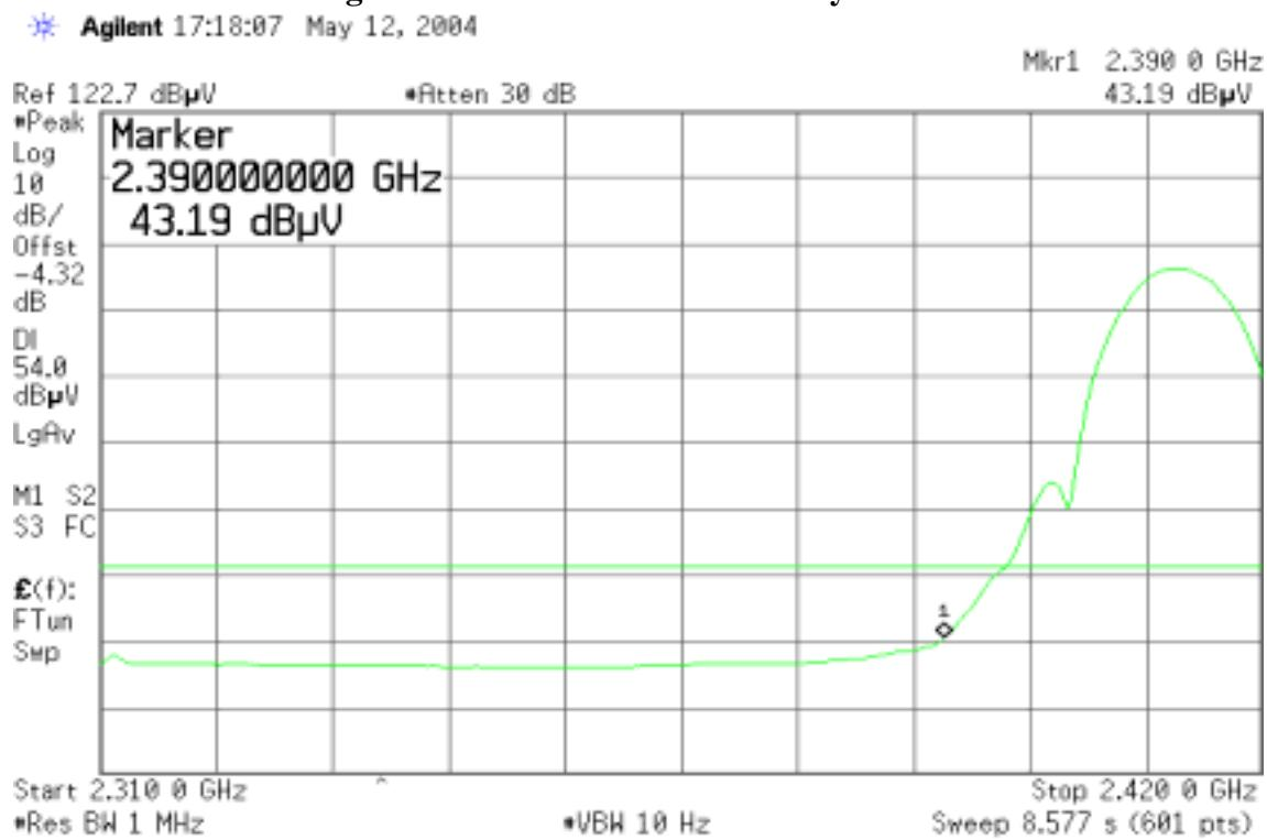
**Band Edges (CH High)****Detector mode: Peak****Polarity: Vertical**
