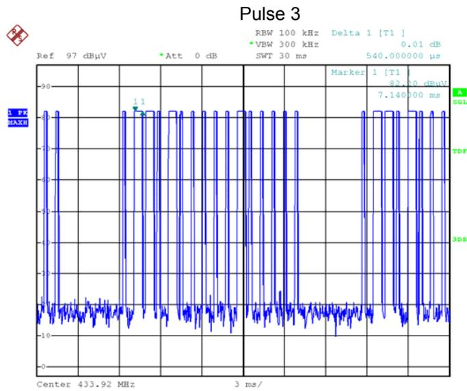
FCC Part15.231 (a) (1) A manually operated transmitter shall employ a switch that will automatically deactivate the transmitter within not more than 5 seconds of being released.
