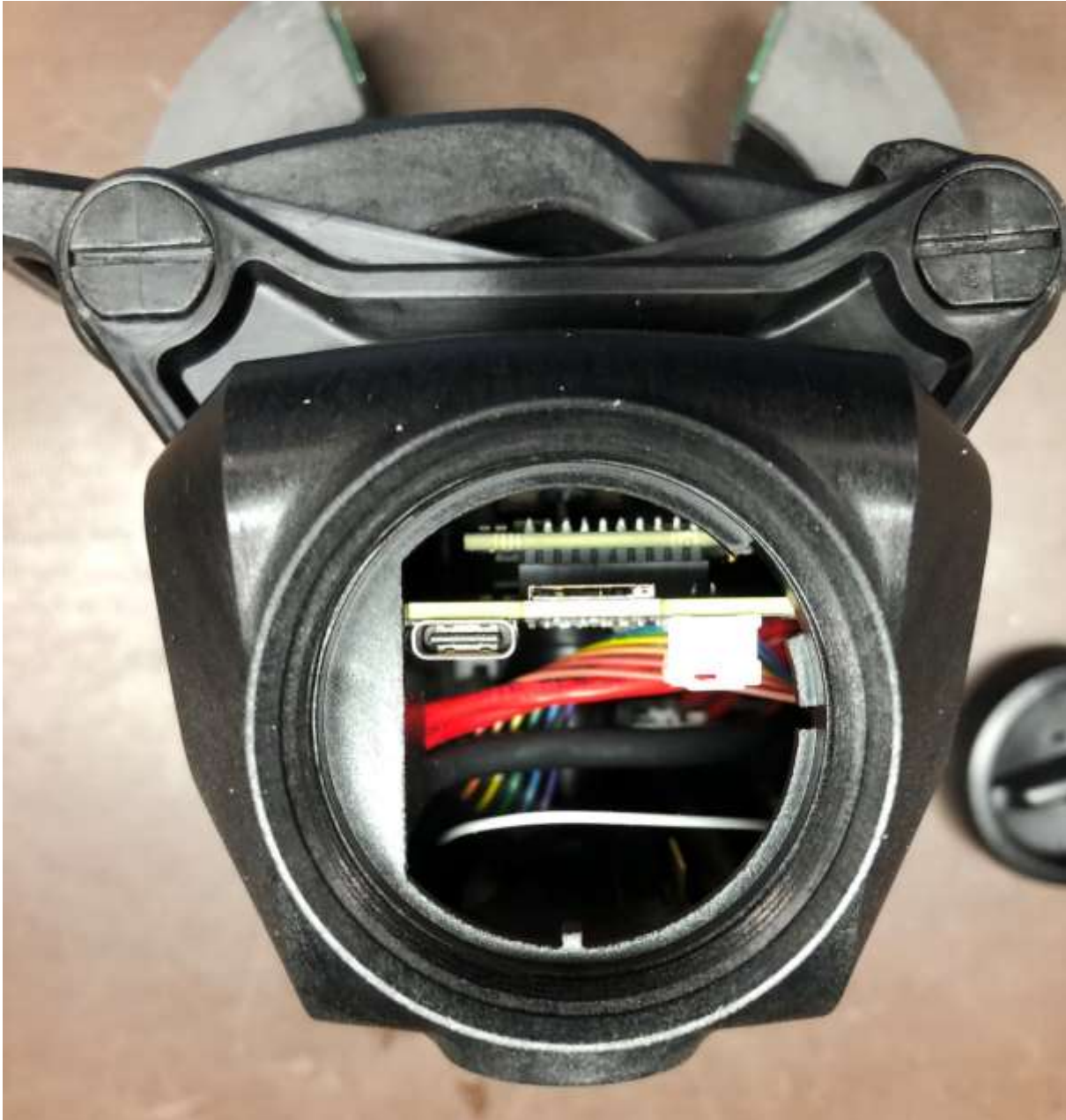
Figure 1: GridAdvisor 3 Internal View With Cover
