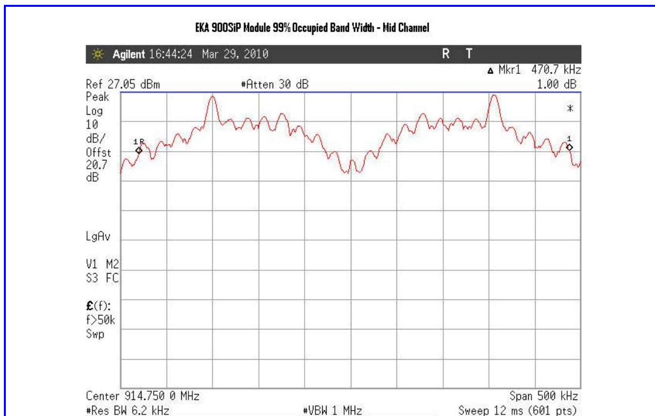
Figure 9: 99% Occupied Bandwidth, Mid Channel
