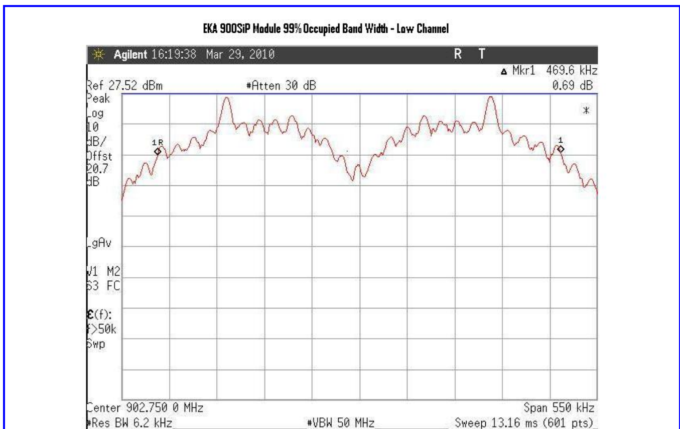
Figure 8: 99% Occupied Bandwidth, Low Channel
