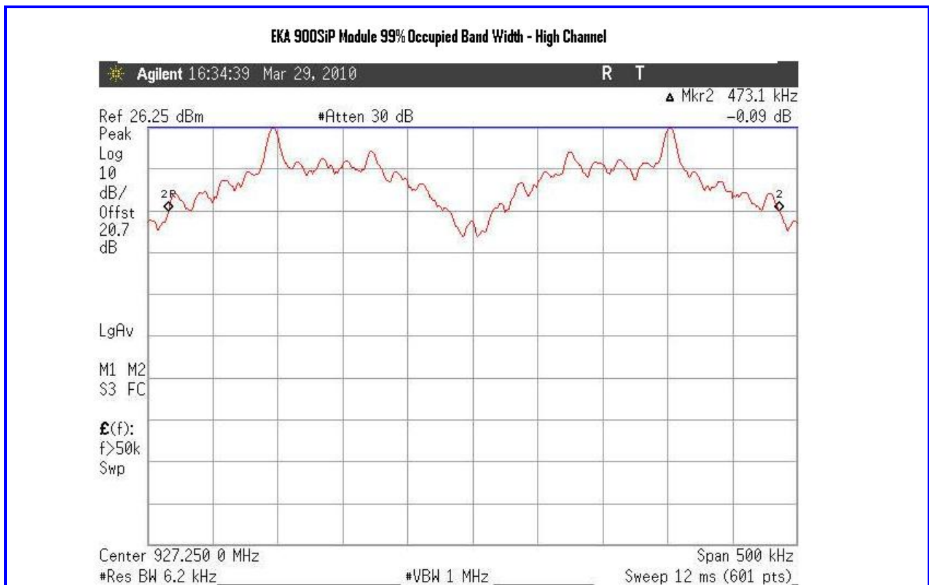
Figure 10: 99% Occupied Bandwidth, High Channel
