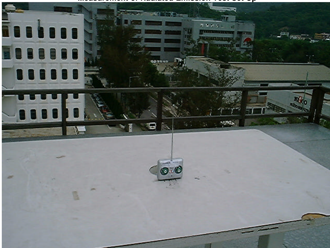
Measurement of Radiated Emission Test Set Up
