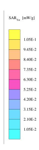
Tilted Right Centre Channel (660) SAM Phantom; Righ Hand Probe: ET3DV6 - SN1529; ConvF(5.20,5.20,5.20) Crest factor: 8.0; Brain 1900MHz:  $\sigma$  = 1.49 mho/m  $\epsilon_r$  = 37.5  $\rho$  = 1.00 g/cm³ Lab Temperature 21.5 deg C, Fluid Temperature 18.5 deg C SAR Drift 3.6% 12/11/02
