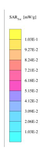
Cheek Right Centre Channel (660) SAM Phantom; SAR Right Ref Probe: ET3DV6 - SN1529; ConvF(5.20,5.20,5.20) Crest factor: 8.0; Brain 1900MHz:  $\sigma$  = 1.49 mho/m  $\epsilon_r$  = 37.5  $\rho$  = 1.00 g/cm³ Peak: 0.107 mW/g, SAR (1g): 0.0586 mW/g Lab Temperature 21.5 deg C, Fluid Temperature 18.5 deg C SAR Drift 8.4% 12/10/02
