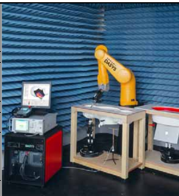
Fig. 5.2 Probe Setup on Robot
