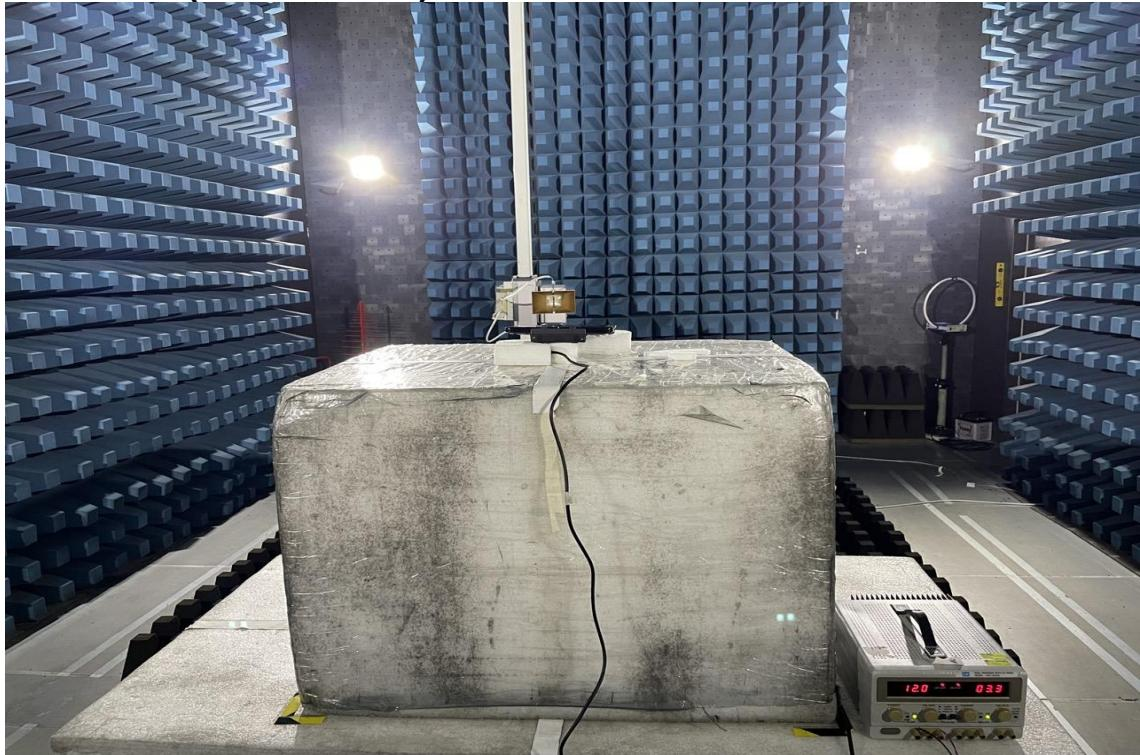
**Conducted Emission Set Up Photo**
