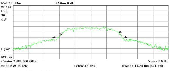
Occupied Bandwidth 1.1297 MHz Occ BW % Pwr 99.00 % x dB -20.00 dB
