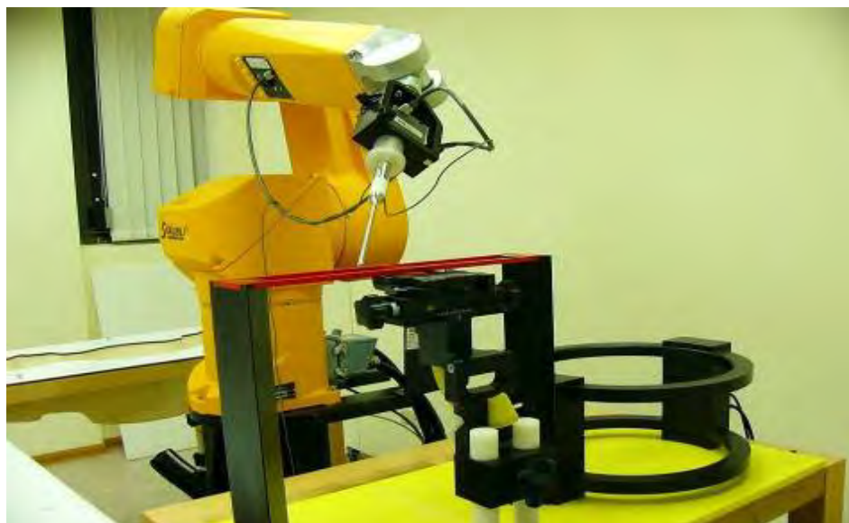
Fig. 1 Photograph of the DASY 5 measurement system
