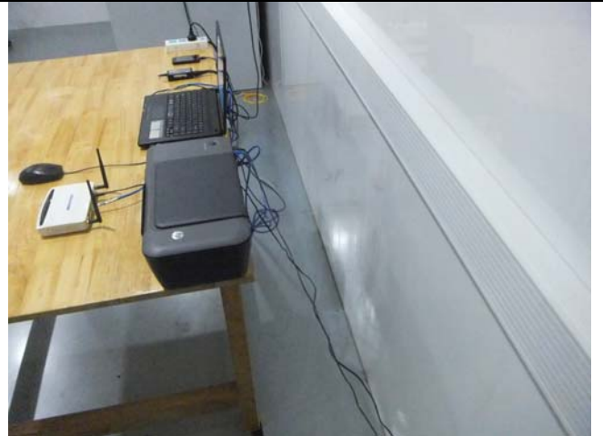
Conducted Emissions Test Setup – Side View
