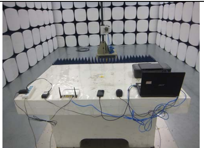
Radiated Emissions Test Setup Above 1GHz
