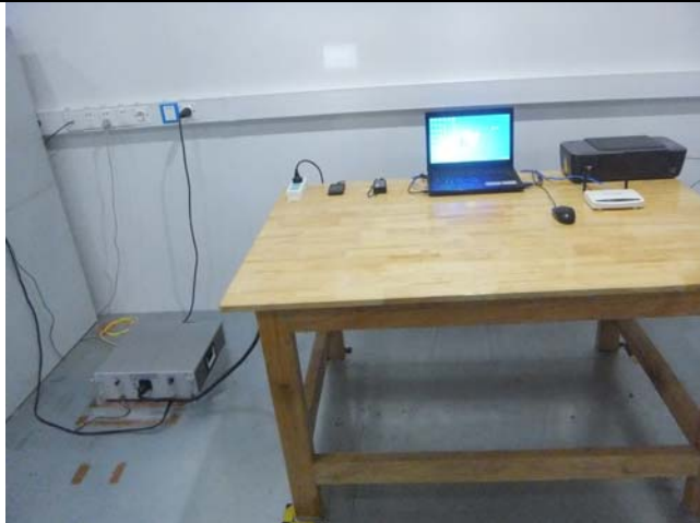
Conducted Emissions Test Setup – Front View
