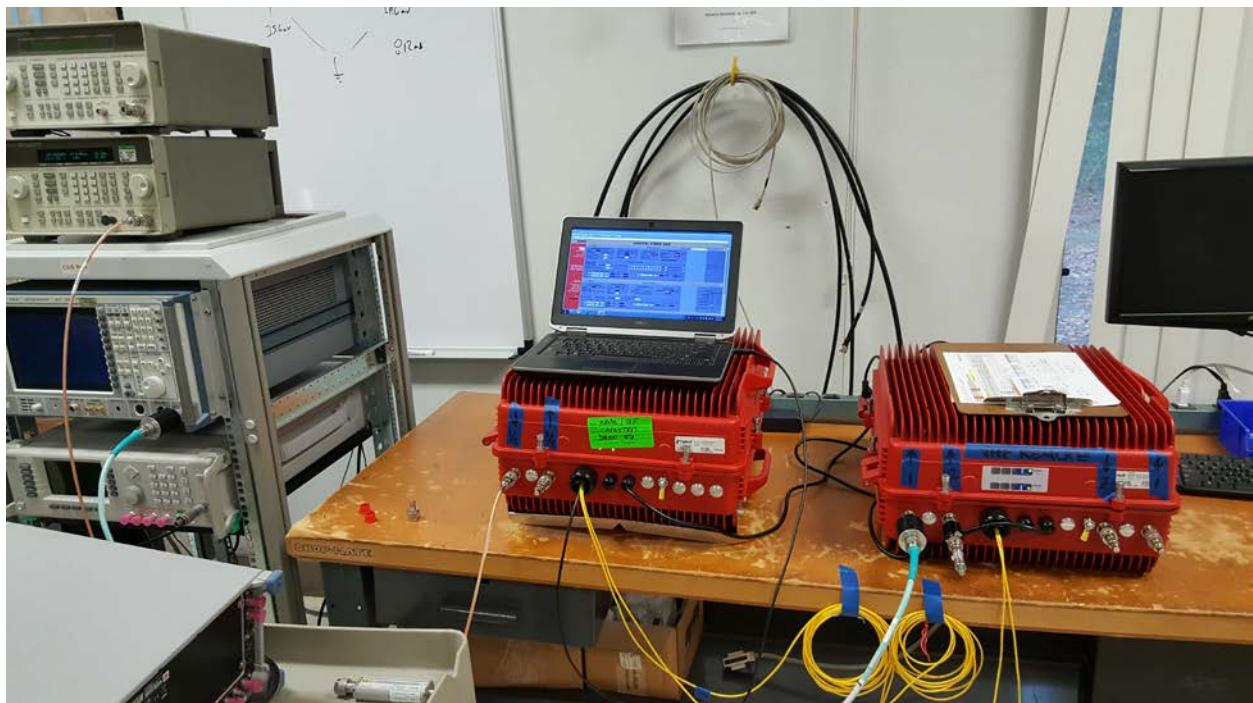
**FIELD STRENGTH SPURIOUS EMISSIONS – TABLE SETUP, FRONT**
