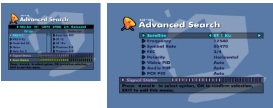
Performs a manual search with the ability to enter PID(Video/Audio/PCR) values. This mode is necessary when you search for the signal that has abnormal service information labels. The setting of the sub items is the same as Manual Search.
