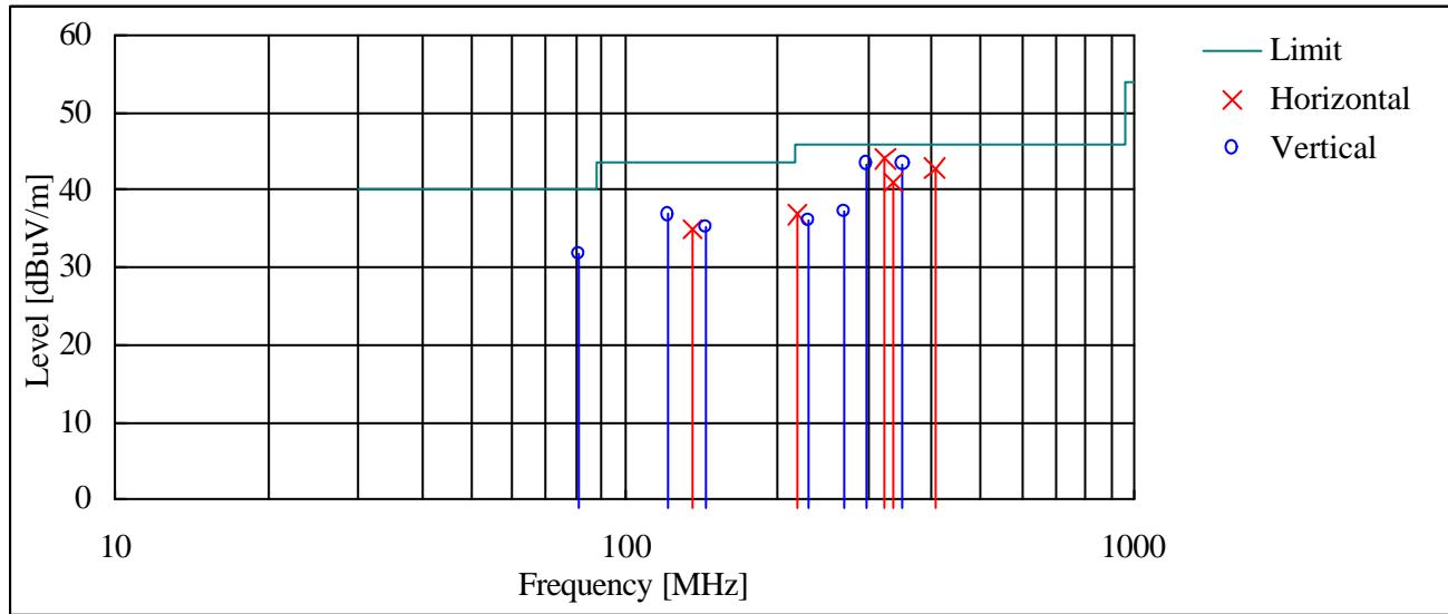
Notes: The test is performed in a distance of 3 m.
