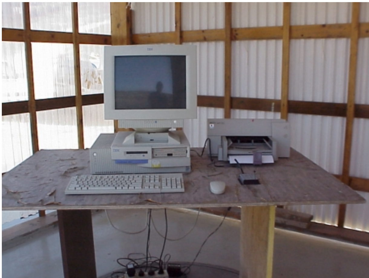
Open field test site Radiated emission test setup
