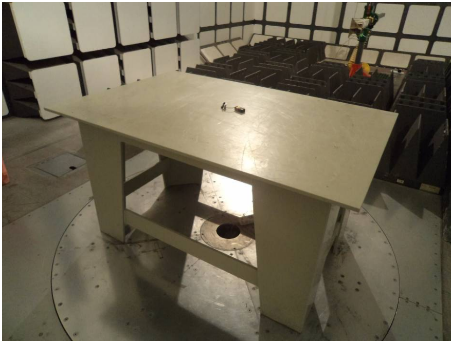
Above 1 GHz: Radiated Emissions View
