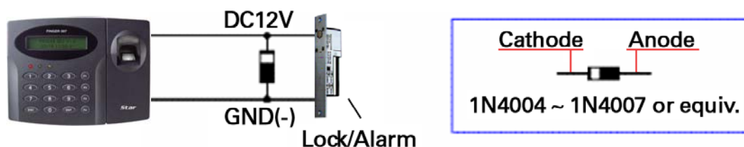
Figure: Reverse Diode Connection
