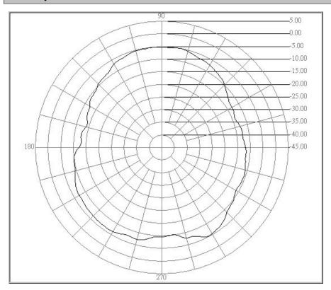
Center freq.(MHz): 2479 Polarization : E Plane
