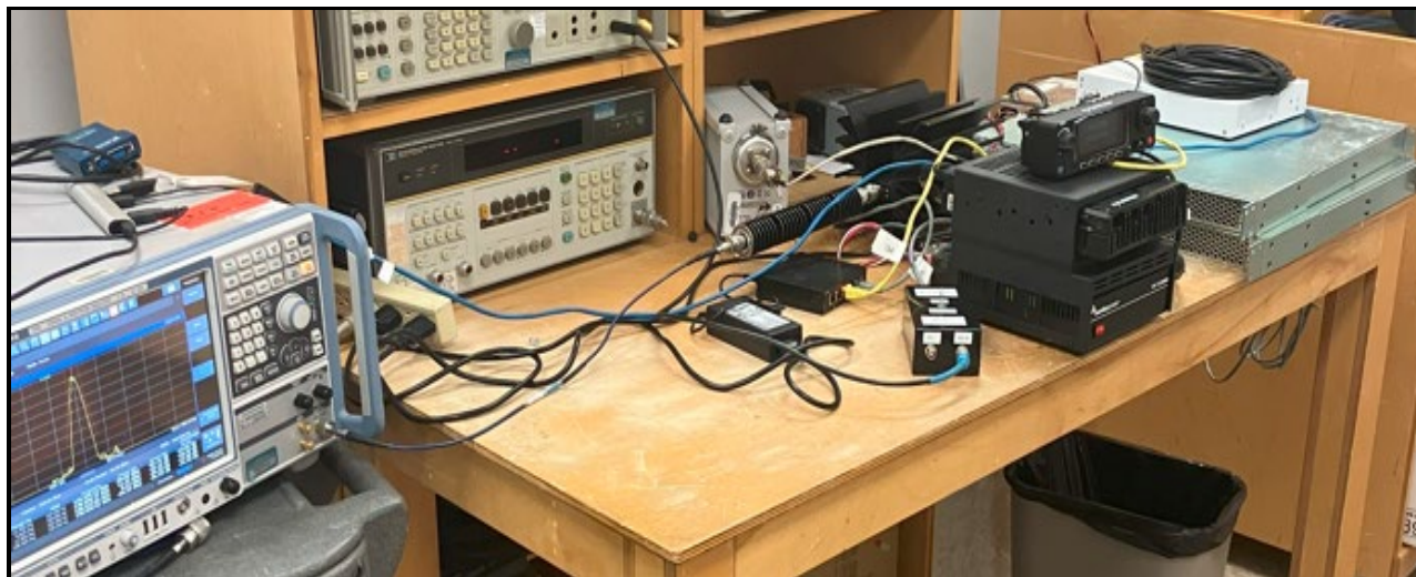
Photograph 5: RF Conducted Emissions
