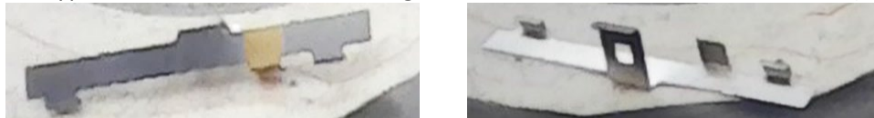
Photo 11: BT/WiFi Antenna , front and back views. Gold area indicates contact point with the spring-loaded pin on Keypad/LCD Solder Side connecting BT/WiFi antenna to PWB BT/WiFi trace (see Photo 9)
