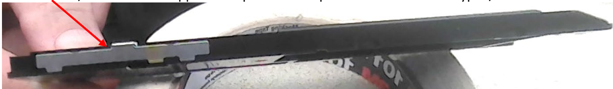
Photo 12: BT/WiFi antenna clipped onto plastic cover piece on back side of Keypad/LCD board
