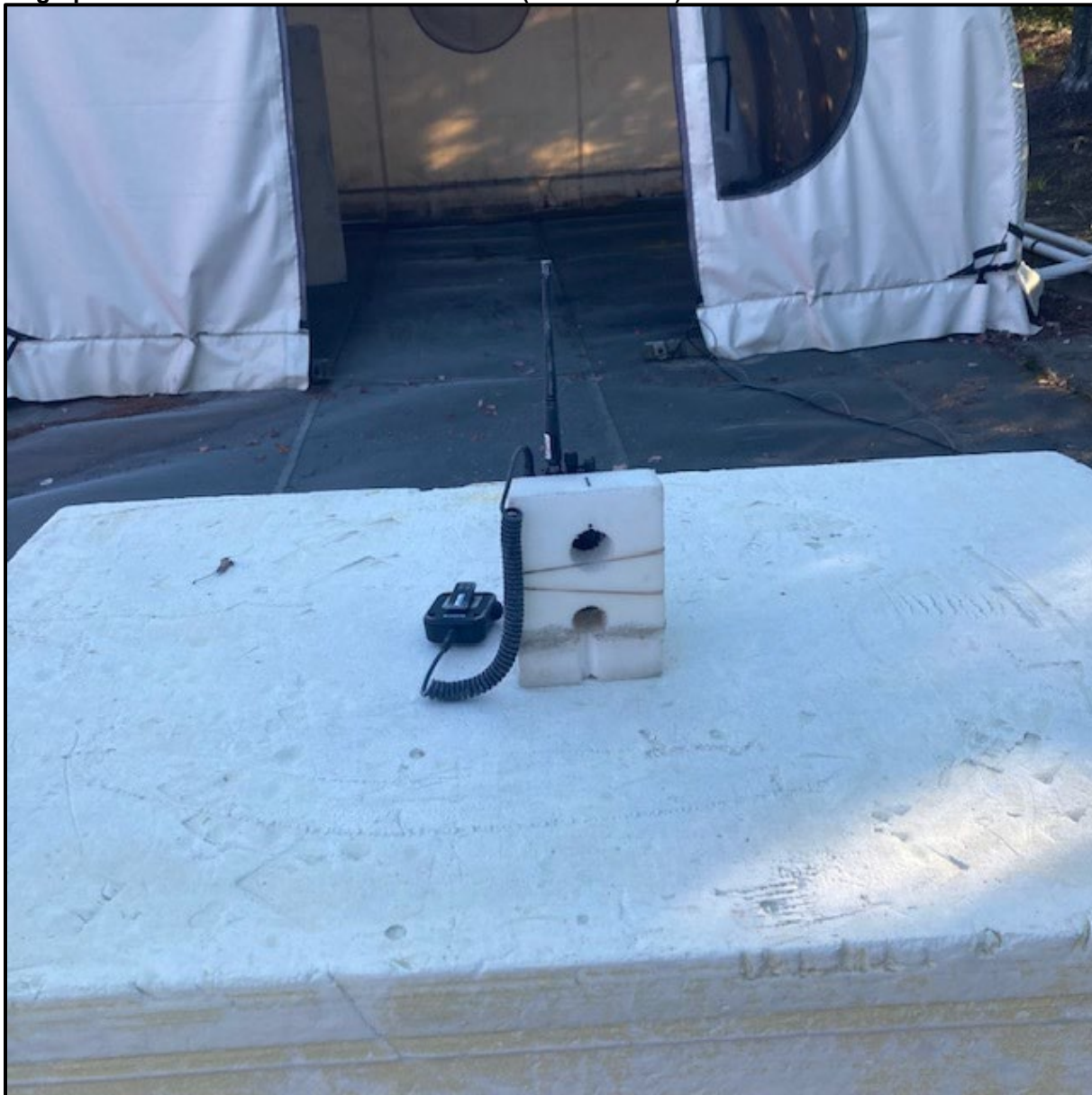
Photograph 2: Radiated Emissions – Back View (Below 1 GHz)
