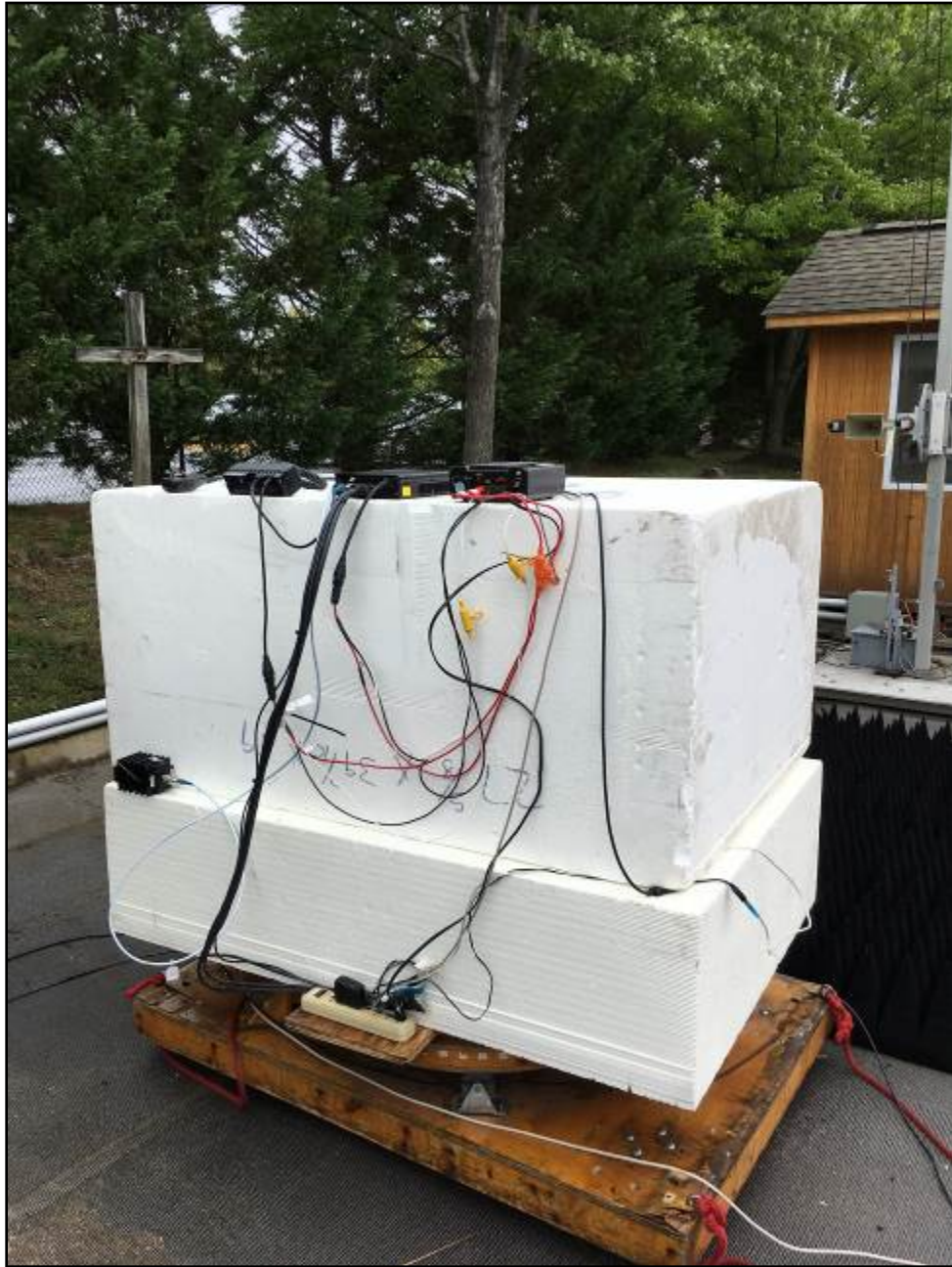
Photograph 2: Radiated Emissions (Spurious/Harmonics) – Back View
