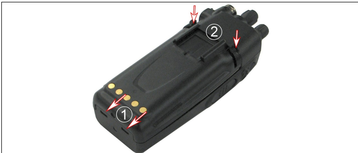
Figure 4-2: Attaching the Battery Pack
