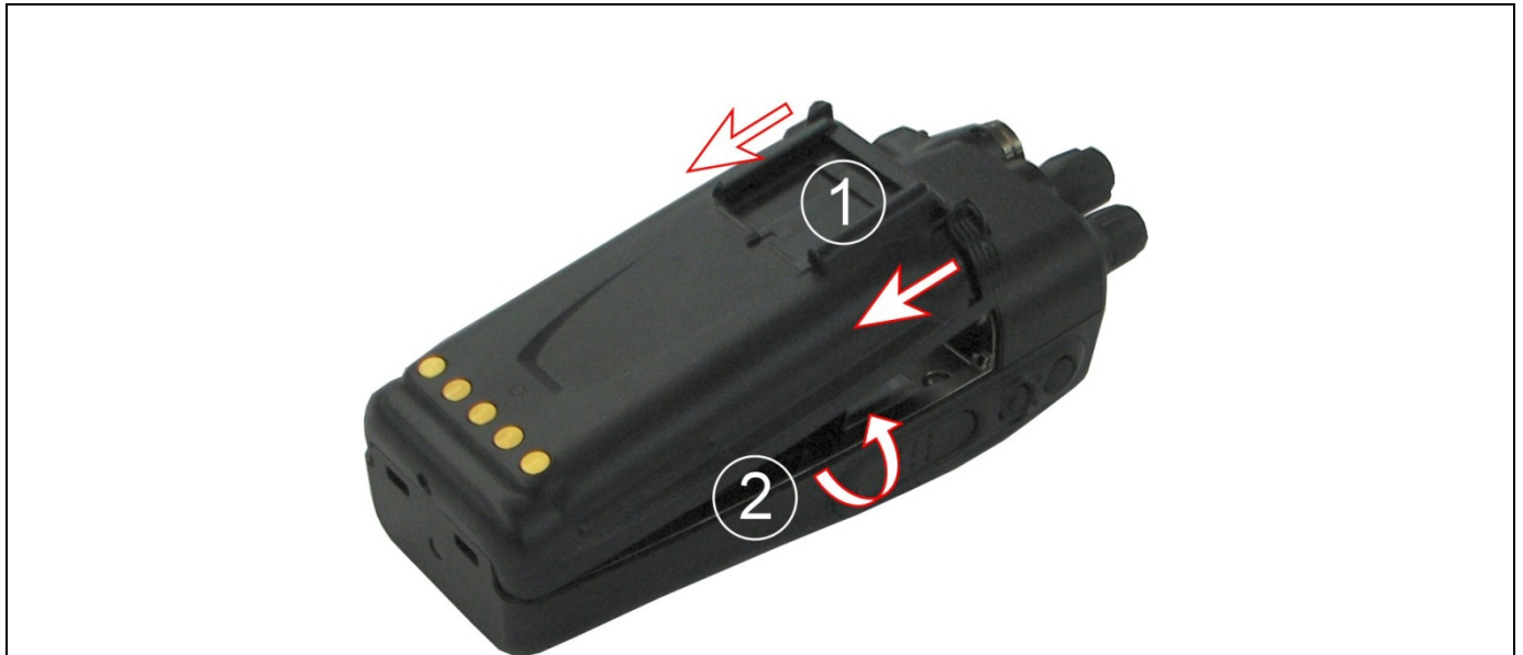
Figure 4-1: Removing the Battery Pack
