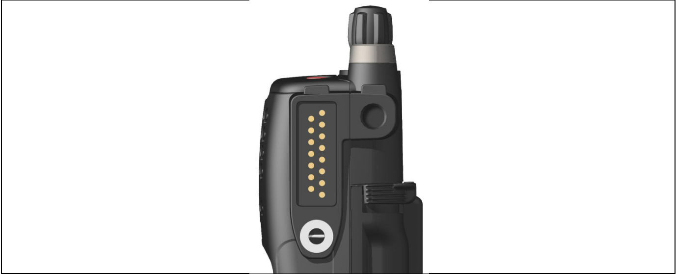
Figure 5-1: XG-25P 15-Pin Universal Device Connector
