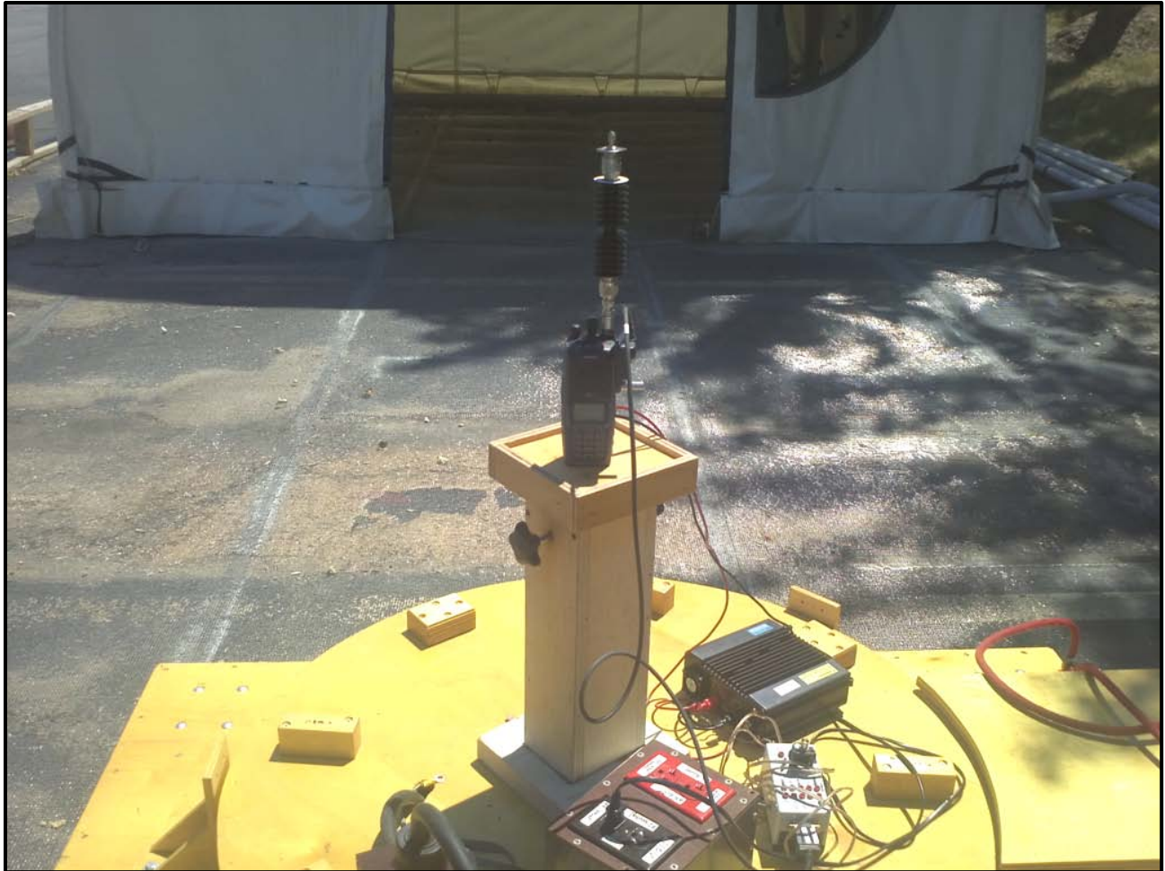
Photograph 5: Radiated Emissions – Front View
