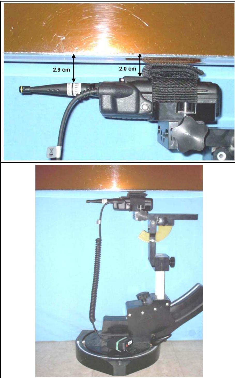
**BODY-WORN SAR TEST SETUP PHOTOGRAPHS**
