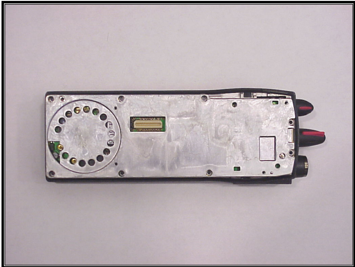
PHOTOGRAPH 8: VIEW OF TOP OF RF SHIELD WITH INTERFACE BOARD REMOVED
