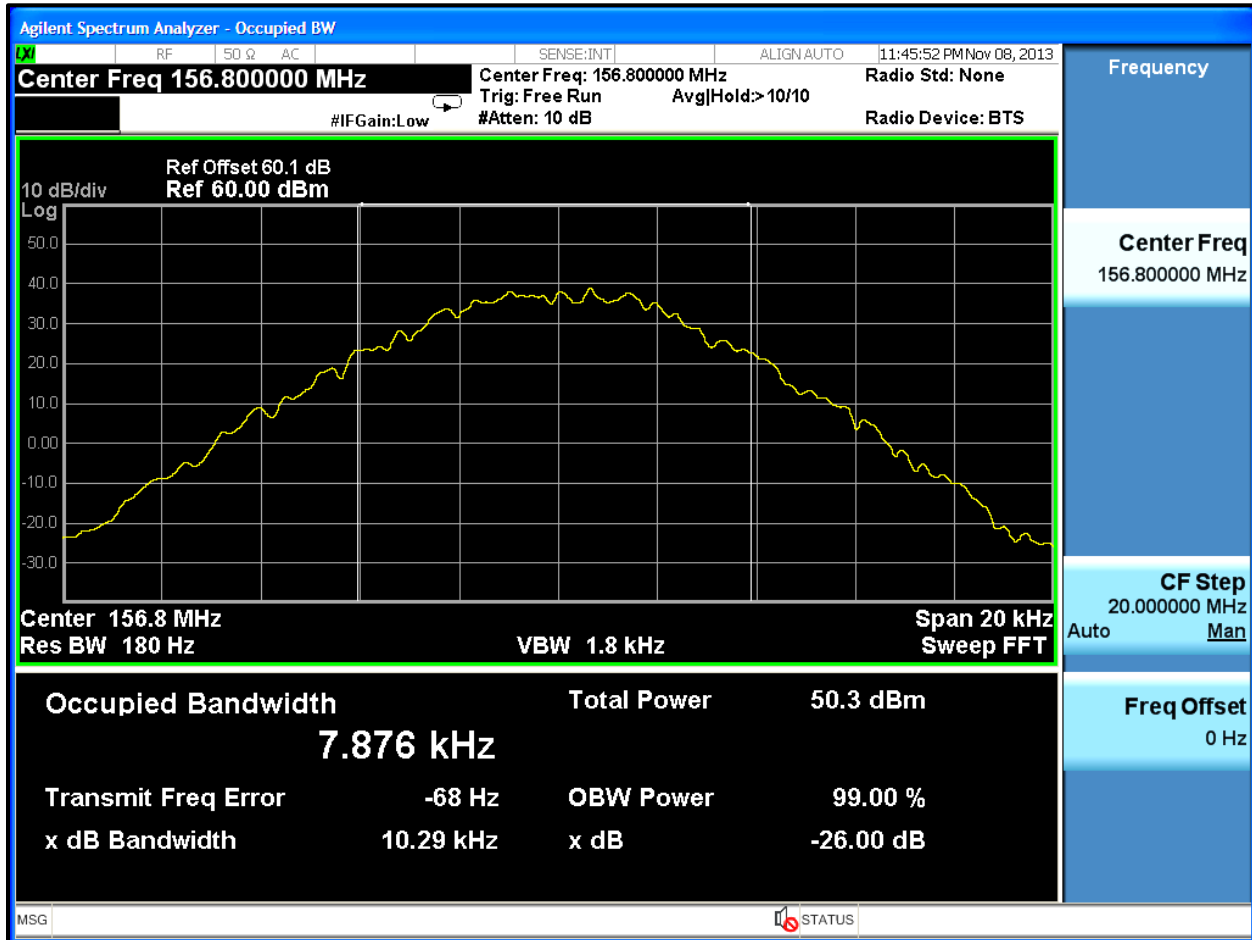
Plot 6-1: Occupied Bandwidth – 156.8 MHz; P25
