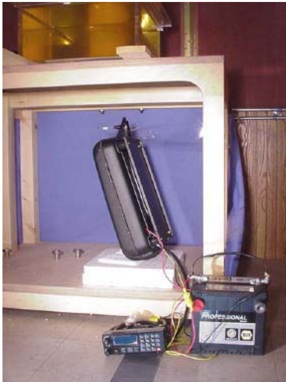
Motorcycle-Mount Unit - SAR Test Setup
