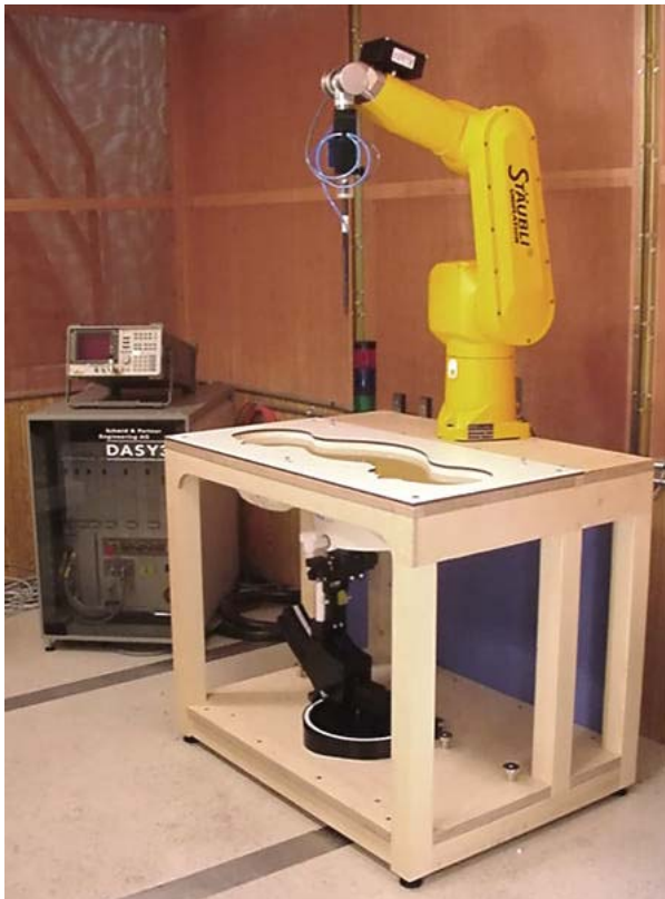
DASY3 SAR Measurement System with SAM phantom
