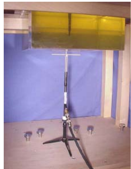
900MHz Dipole Validation Setup
