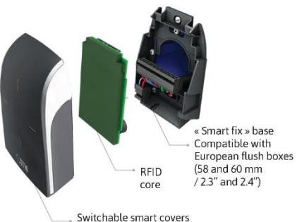
Scalability is a specific feature of the Architect® Blue series. Each reader is composed of three parts: one switchable cover, one RFID core and one smart mounting plate. You can upgrade functionalities and security levels by switching the cover and/or adding a biometric module.
