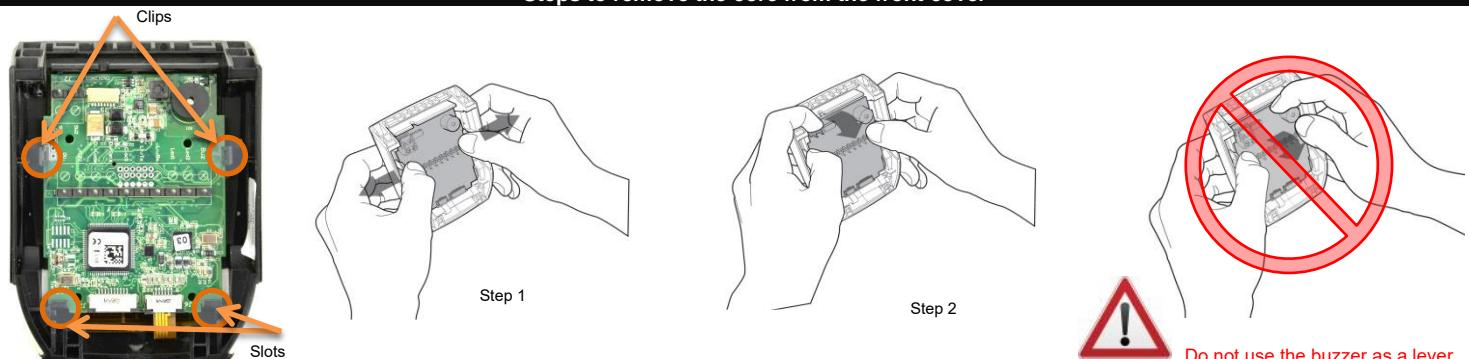
Procedure to install the core into the front part
