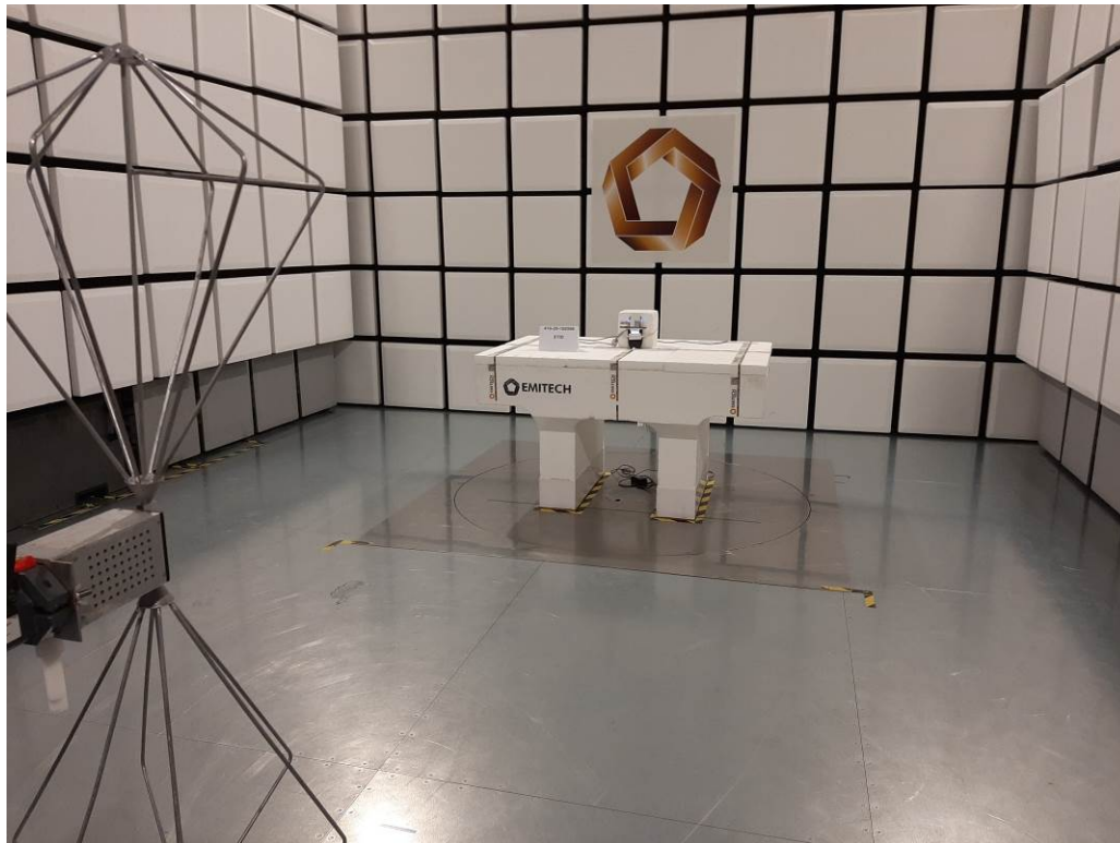
TEST SETUP PHOTO(S) RADIATED EMISSIONS (30MHZ-200MHZ)
