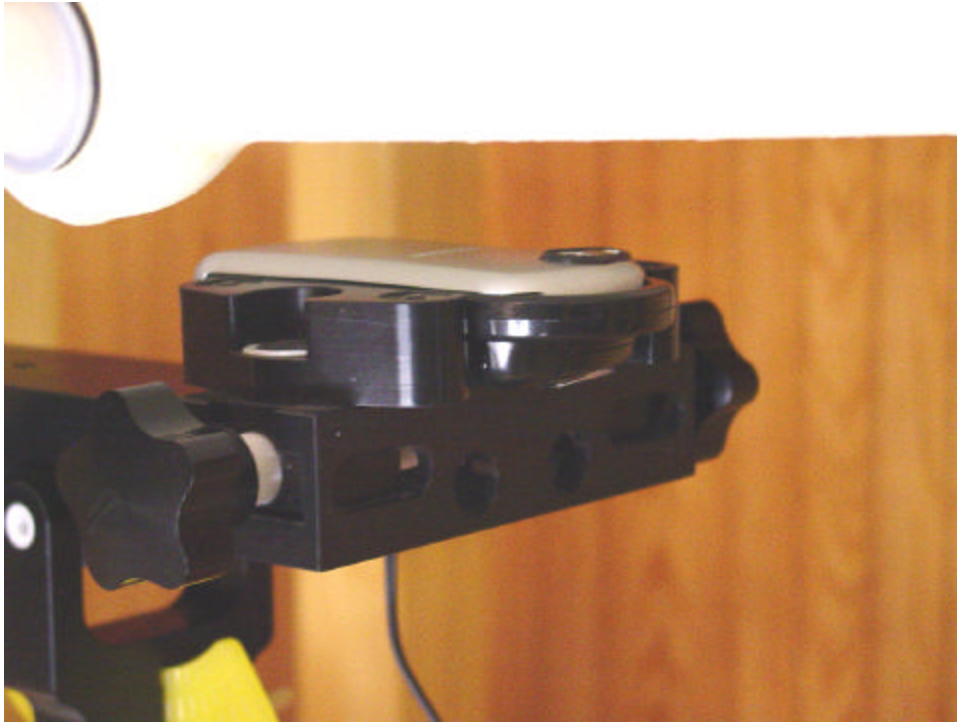
Figure 12.4 body SAR setup (with 25mm air separation)
