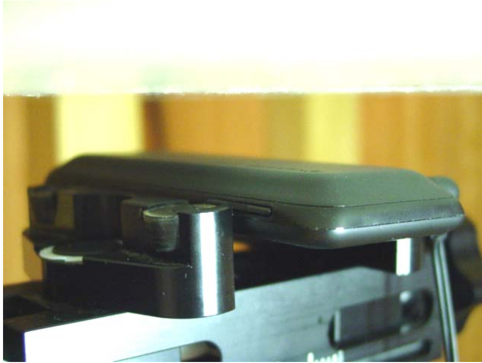
Figure 9E.3 Body SAR setup (15mm Air Separation)
