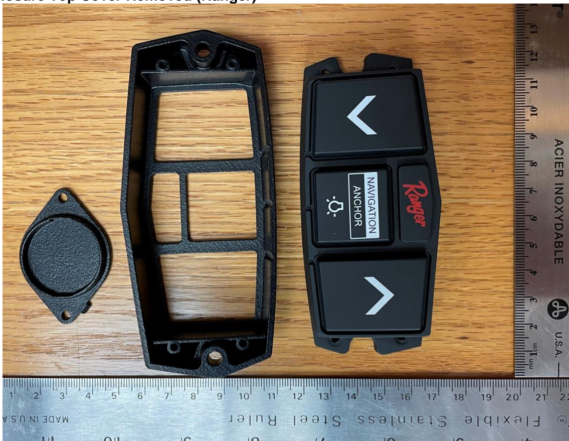
Enclosure Top Cover Removed (Ranger)
