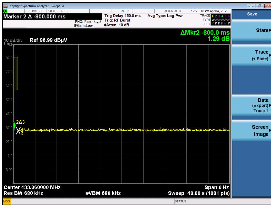
Screen Captures from the spectrum analyzer: Silent Time
