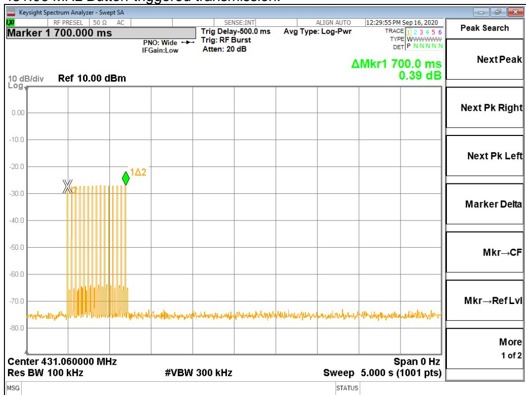
433.06 MHz Button-triggered transmission:
