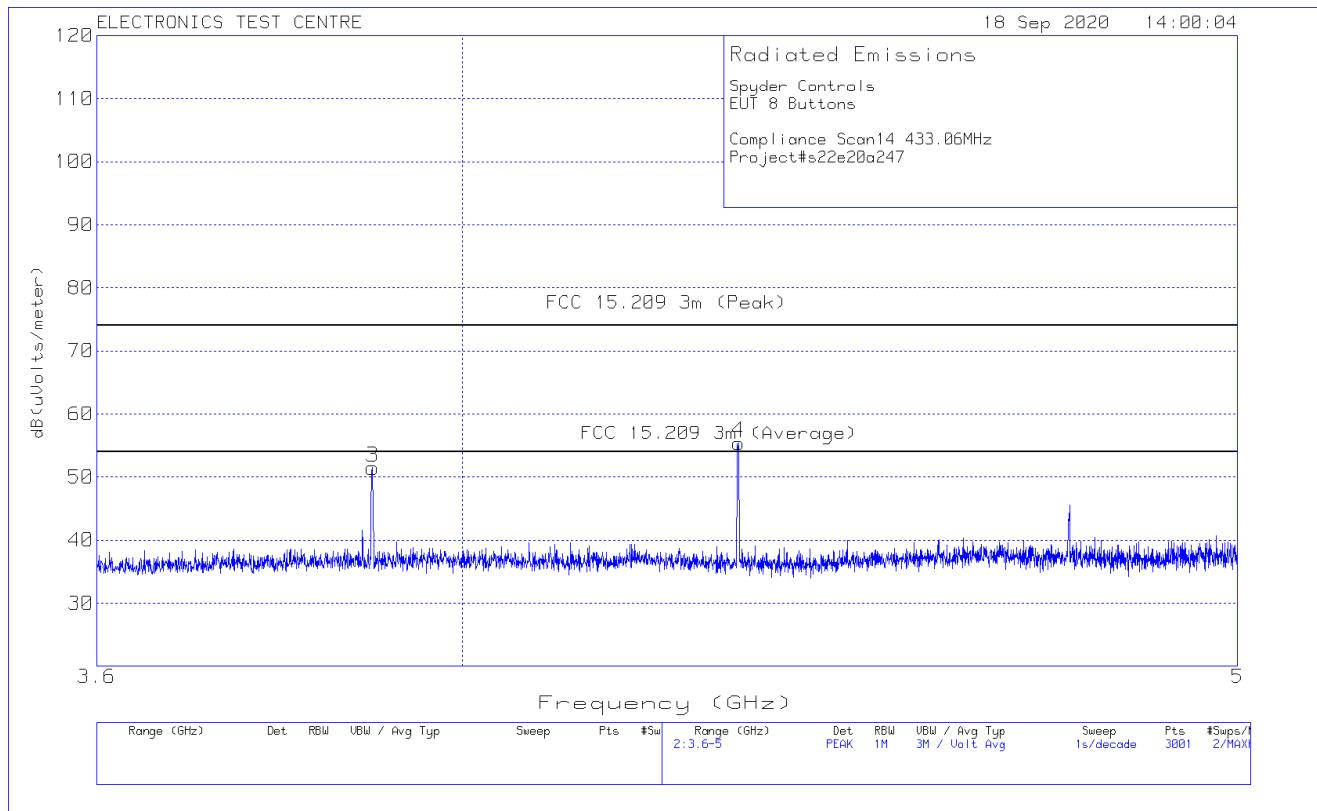
**Plot of Radiated Emissions: Horizontal polarization (Ambient)**
