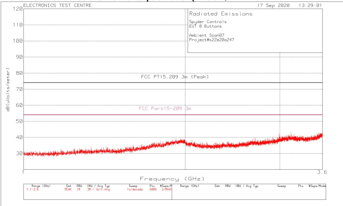
**Plot of Radiated Emissions: Vertical polarization (Ambient)**
