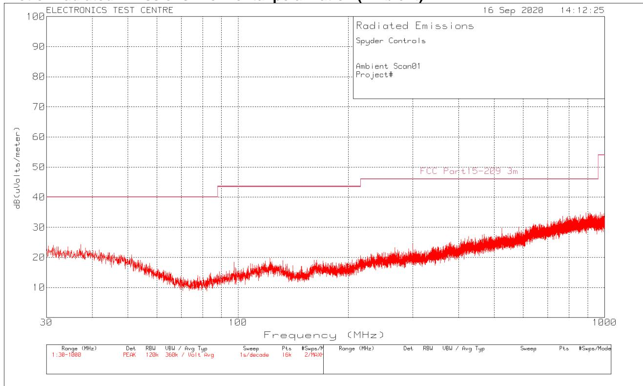
**Plot of Radiated Emissions: Vertical polarization (Ambient)**
