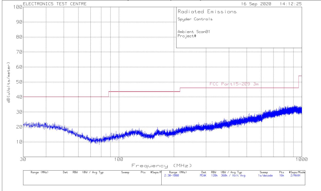
**Plot of Radiated Emissions: Horizontal polarization (Ambient)**
