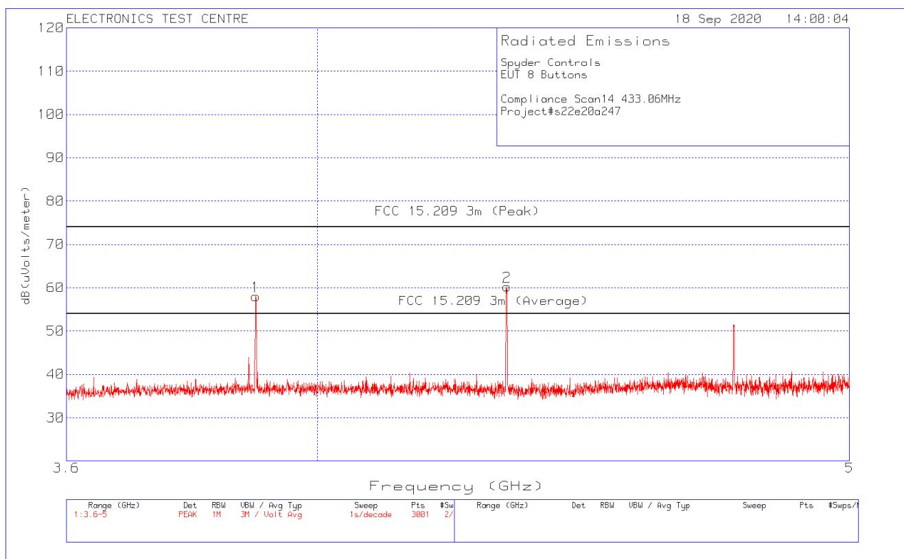
**Plot of Radiated Emissions: Vertical polarization TX@433.06 MHz**
