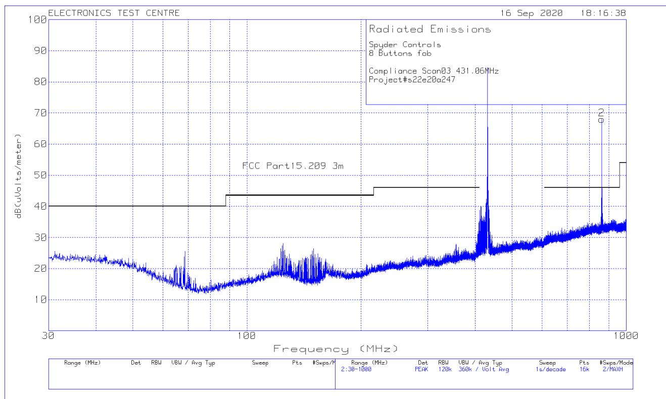
Plot of Radiated Emissions: Horizontal polarization [Tx@431.06 MHz](#)
