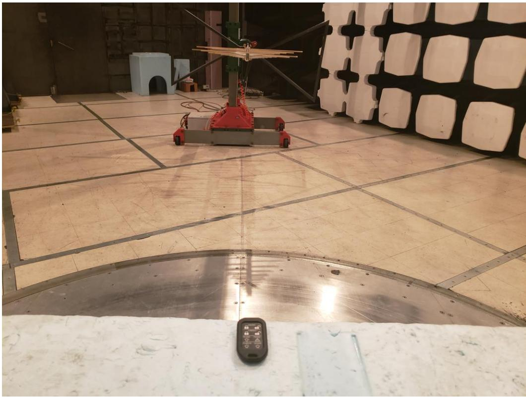
**Radiated Emission 30 MHz to 1 GHz Test Setup:**
