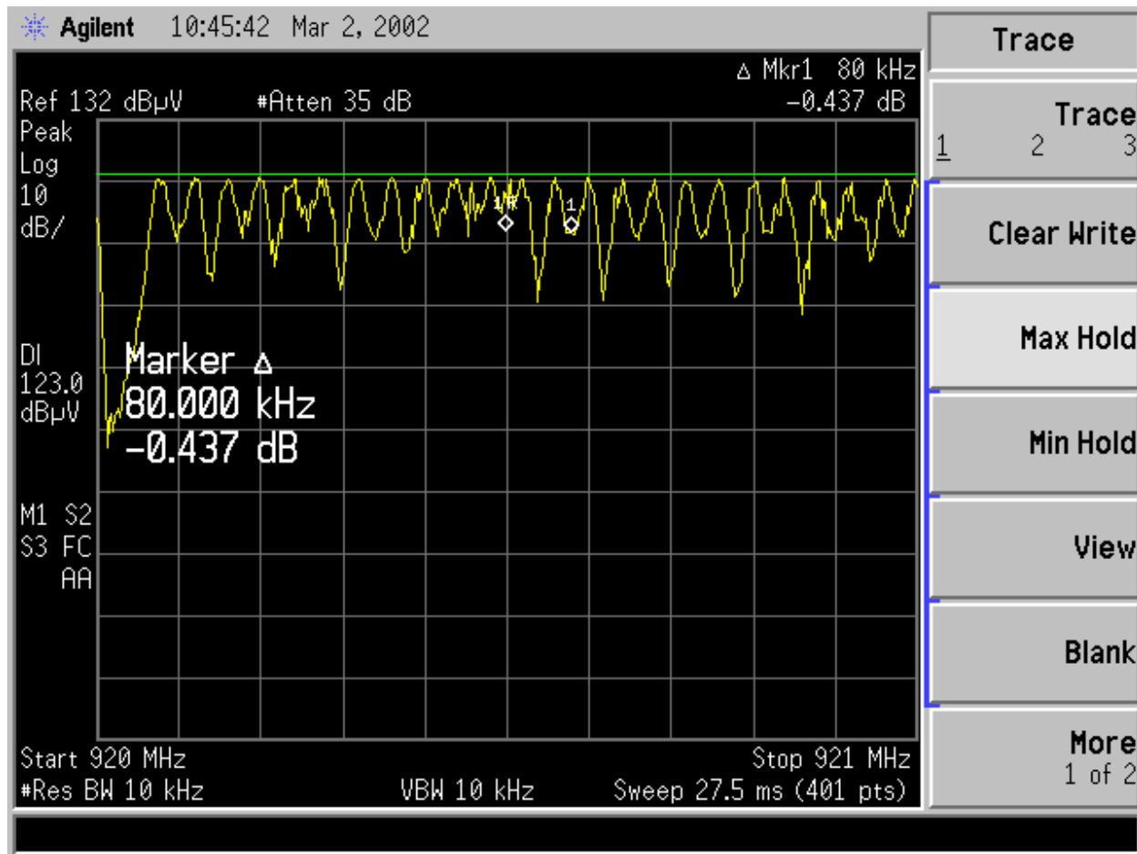
The channel separation was 80 kHz, which is larger than 65 kHz. The EUT meets the requirements.
