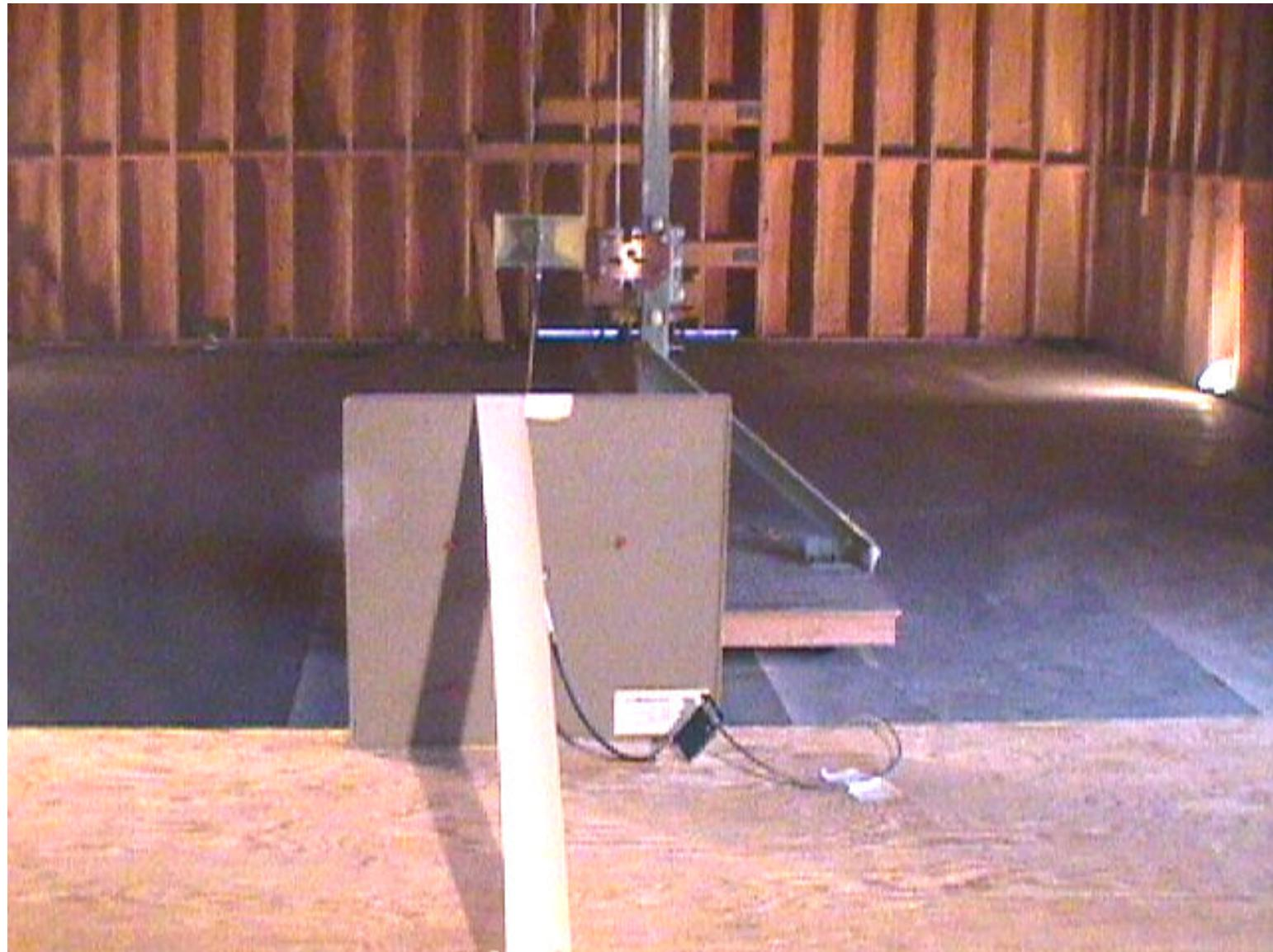
**ANNEX 2 - TEST SETUP FOR TRANSMITTER RADIATED EMISSIONS
