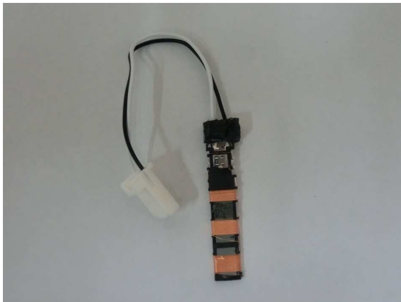
Figure 8.16 LF-antenna InF,InR (G8D-841M-ANT) internal (back view)
