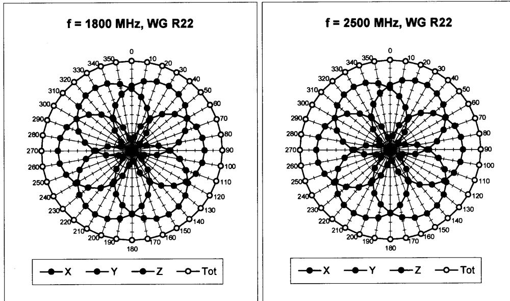
**Isotropy Error ( $\phi$ ),  $\theta = 0^\circ$**
