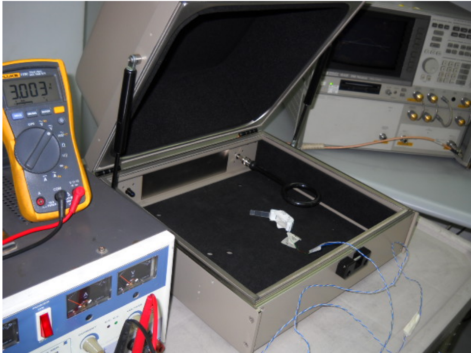
Photograph No.4 Setup for occupied bandwidth measurements
