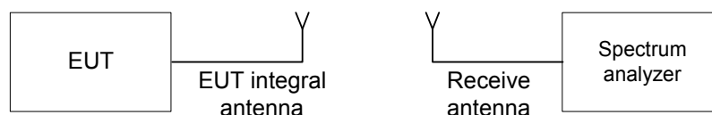
Figure 7.1.1 Setup for transmitter shut down test
